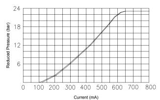
Curve is attained with SAE 40 - Grade oil @ 50°C
