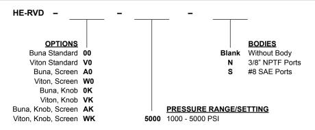
Note: use screen only if flow direction is from (1) to (2).
