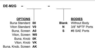
Note: use screen only if flow direction is from (1) to (2).
