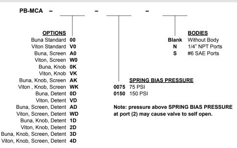
Note: use screen only if flow direction is from (1) to (2).
