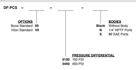
Differential Pressure Across External Controlling Orifice
