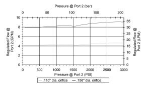
Priority port (2) load: 1500-1700 psi, .156" dia orifice, 15 gpm supply not intended for differential pressure > 1500 psi port (4) to port (3)
