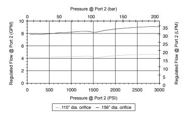
Priority port 2 load: 1500 - 1700 PSI, .156" dia orifice, 15 GPM supply not intended for differential pressure > 1500 PSI port 4 to port 3
