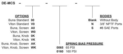
Note: use screen only if flow direction is from (1) to (2).
