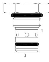
7 size, 5/8-18 thread, "Mini" series, direct acting check valve.
